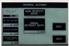
The lead tech notes that the control's "auto setpoint" feature allows the operator to easily establish noncritical stroke parameters such as top of stroke and slowdown setpoints visually. The operator simply jogs the press to the desired position, selects the setting parameter, and selects auto setpoint. The control then automatically stores the actual position as the setpoint for that parameter, eliminating the need to take measurements.
